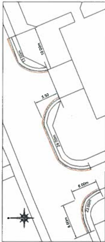
Road Marking : Location 2 Scale 1:250
